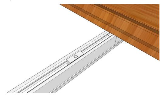
2.2: Then place the plate with the fastener installed flat, the position of the fastener can be pressed heavily to make the spike position better.
