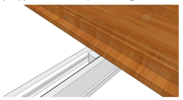
2.3: Just place a limit clip on each board, and the position can be centered.
